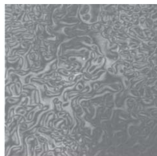
Fig. 3. a) DSC curves of compound 4e : 1 – first heating; 2 – first cooling; b) Optical texture of compound 4e , 184°C, first heating
